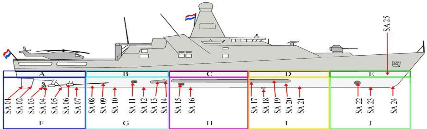
Gittenberger et al. (2018) when assessing hull-fouling on naval ships of the Netherlands, the hull surface was divided in various zones where different biofouling communities were expected to be recorded. All niche areas were also identified and sampled. Biofouling species diversity differed strongly across niche area. Some niches in general form a higher risk of NIS being present than others. This will be taken into consideration in the Baseline Study Design
