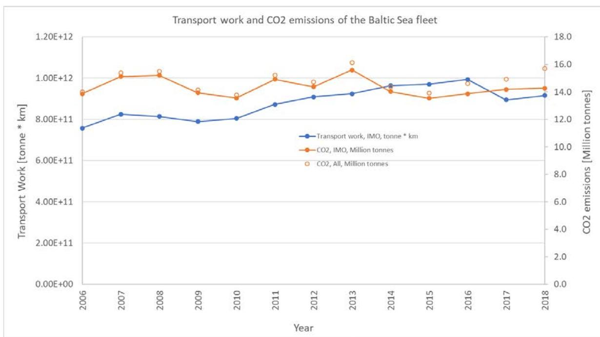
**Figure 2** Transport work and CO<sub>2</sub> emissions of the Baltic Sea fleet. Transport work (blue line and blue symbols) has increased by +12.5% during the last decade. The emissions of CO<sub>2</sub> (orange line, orange symbols) have been reduced by -6.2% during the same period. This translates to 20% energy efficiency improvement in the Baltic Sea area. The open symbols indicate CO<sub>2</sub> emission totals including the non-IMO regulated traffic.
