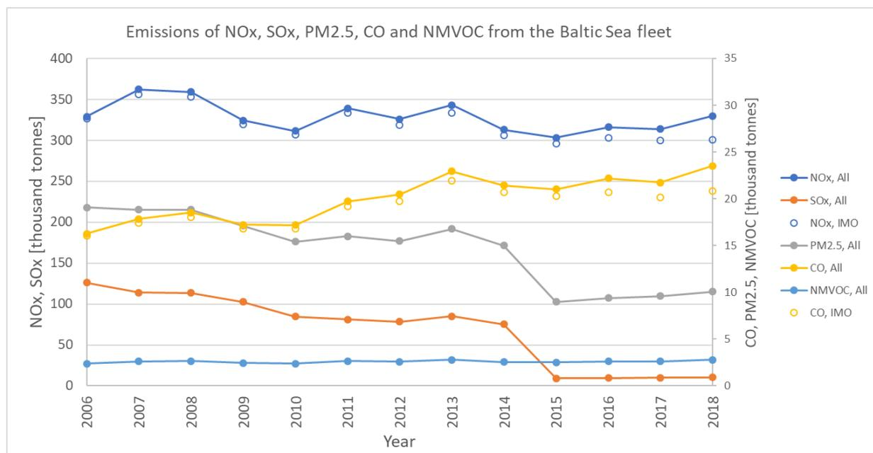
**Figure 1 Emissions of NO<sub>x</sub>, SO<sub>x</sub>, PM<sub>2.5</sub>, CO and NMVOC from ships in the Balti Sea during 2008-2018. Significant decreases in SO<sub>x</sub> and PM<sub>2.5</sub> are results of regulatory changes concerning the maximum Sulphur content of fuel. Colored symbols depict total emissions from all vessels with an active AIS transceiver, empty symbols indicate the contribution from IMO-registered ships only.**
