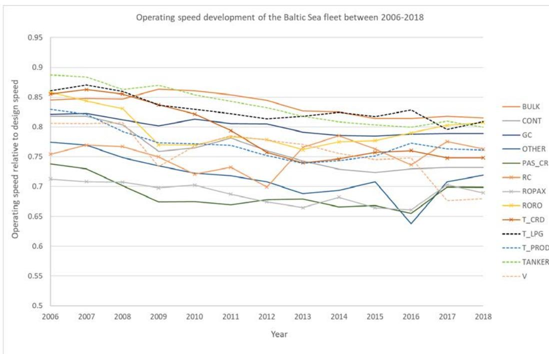
**Figure 4** Operating speeds of various types of ships in the Baltic Sea fleet. The numbers presented report the relation between average cruising speed to the design speed of each class. This figure illustrates a widespread use of slow steaming across all ship types in the Baltic Sea fleet.
