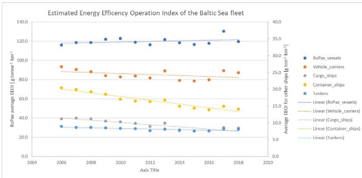
**Figure 3** Development of estimated EEOI over the period 2006-2018. Values for RoPax vessels are given in left axis whereas the values for other ship types are indicated on the right axis.
