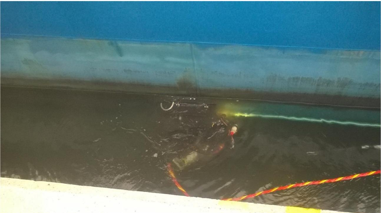
**Figure 2. A diver is cleaning the hull with the cleaning machine unit.**
