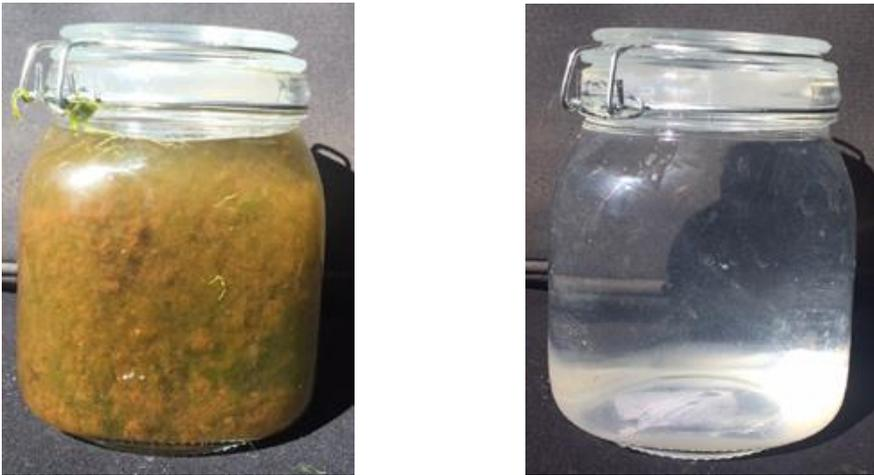
**Figure 3. A) Process water containing algae, barnacles etc., B) Purified process water.**
