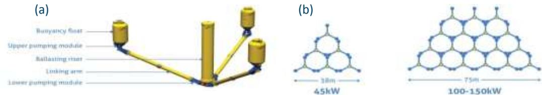
Figure 1 Schematic drawing of the Albatern WaveNET (a) Single SQUID device (b) extended WaveNET array with approximate dimensions and expected power generation. ([www.albatern.co.uk/wavenet](http://www.albatern.co.uk/wavenet))
