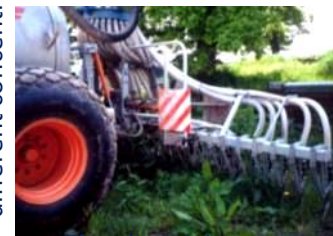
The slurry injector.
