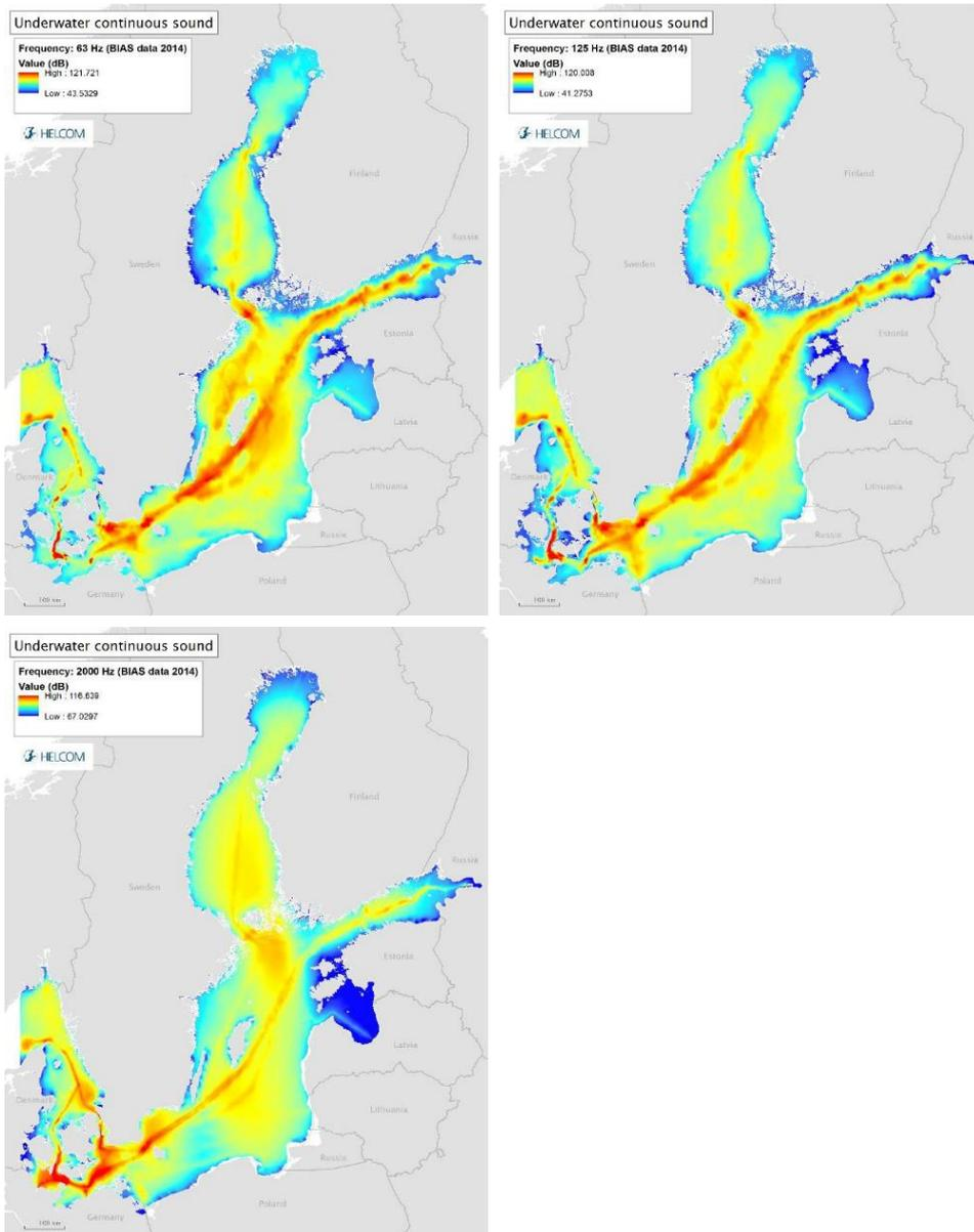
Figure 4.4.1. Soundscape maps in the Baltic Sea, showing underwater continuous sound at 1/3 octave frequency bands of 63 Hz, 125 Hz and 2000 Hz. Areas with high sound level overlap clearly with the location of major shipping routes. The sound produced
