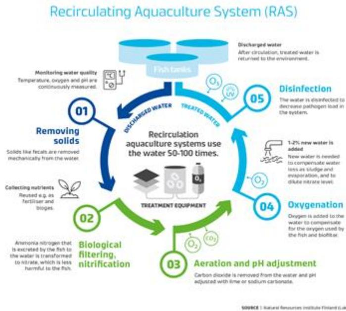
**Figure 2.** Typical water treatment steps in within a RAS farm.
