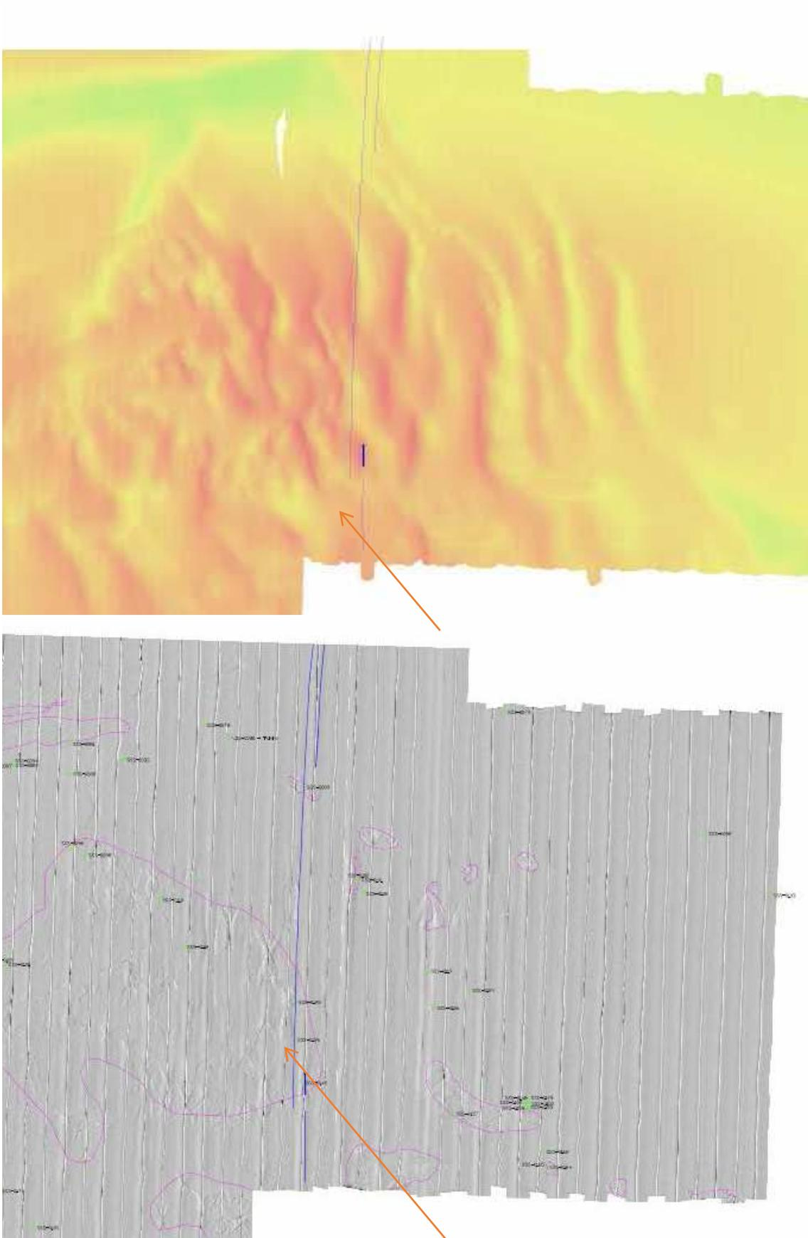
*Image 5 and 6: Bathymetric and side scan sonar images showing two parallel cables (arrows) in the Plantagenetgrund NW sand extraction area (corresponding to the full part of the vertical red line in Image 4)*
